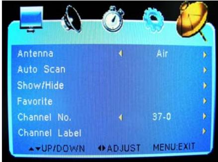
First, make sure your monitor antenna is showing "air" mode for Modulus, Canatrans, or other UHF Transmitters. "CATV" antenna is only to be used for CATV Channel 59 transmitters.
