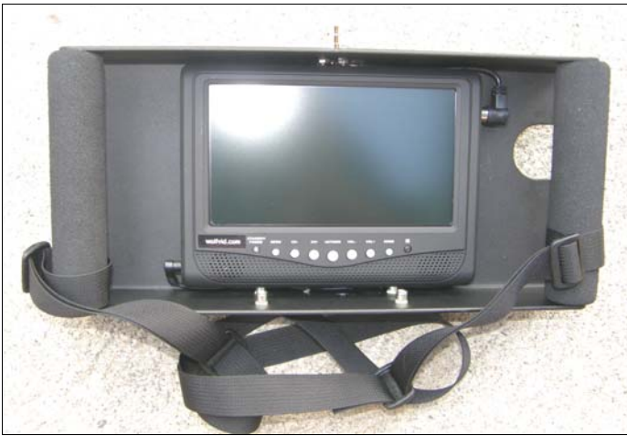
7" or 10" handheld with tuner and 6 hr battery
